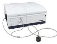
Model F-7100 Fluorescence Spectrophotometer (Optical fiber accessory installed)
