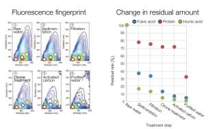
The residual fraction of organic substances that cause bad odors, in addition to trihalomethanes, can be ascertained by measuring the fluorescence fingerprint following each treatment step in a water purification plant(PARAFAC analysis).
