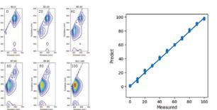
While an ordinary calibration curve is prepared using a single wavelength, high precision quantitative determinations can be made using multiple wavelengths (PLS-LASSO regression).
